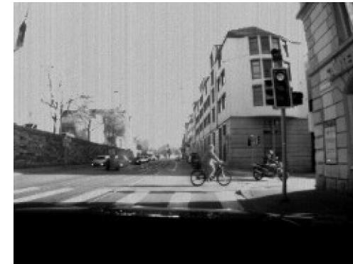
Gray-level frame and triggered events. Where brightness variations don't occur, no events are triggered!
